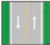
Two direction roadway, passing permitted
