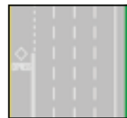
One direction roadway, separating express lane or carpool lane from general lanes—crossing prohibited
